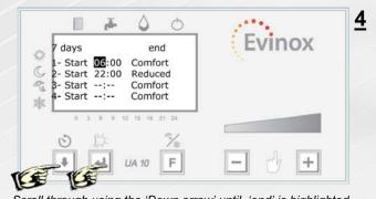
Scroll through using the 'Down arrow' until 'end' is highlighted and press 'ENTER' to exit the screen
